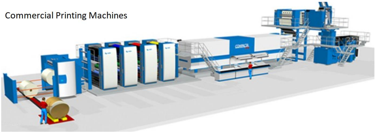
Fig. 3- Commercial printing machines have web as the master motion reference axis, and every station is electronically geared as Slave axis, some stations with registration sensor.
