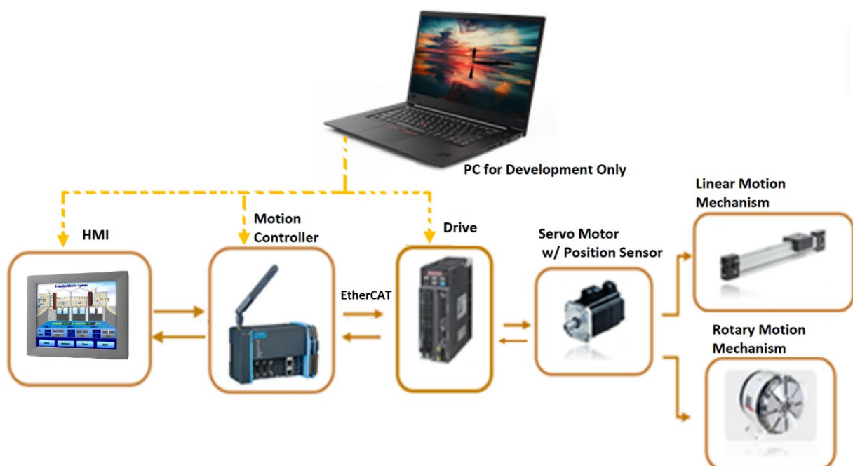
Fig. 1- Components of a single axis servo motion control system
