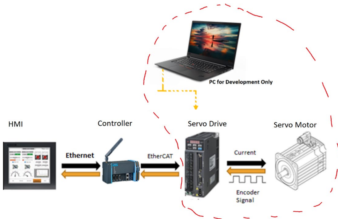
Fig. A-1: A single axis servo motion control system: servo motor, drive, controller, HMI for normal operation. A Laptop PC is used for offline application development purpose.
