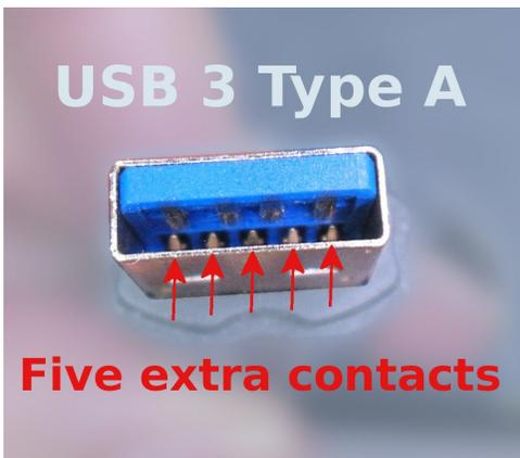
To get more speed, USB 3.0 added 5 more wires to the connectors. The Type-A connector looks the same, but there are 5 more connections deep inside. It might sport the SS trident logo on the right. Although you've probably used USB 3 flash drives that fit this connector and take advantage of the extra speed, you may have never seen a "SuperSpeed" cable with the end shown below.
