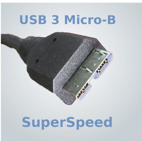
This cable with this Type Micro B connector on one end and a Type A on the other is a "SuperSpeed" cable capable of 5Gbit/s and 10Gbit/s, depending on the age of your devices. Cables under 1 meter long that bear the older SS trident logo are just as good as newer cables with the SS 10 logo. The protocol changed to get the extra speed, but the cables are the same. These cables are seldom used except on external disk drives which need the extra speed.
