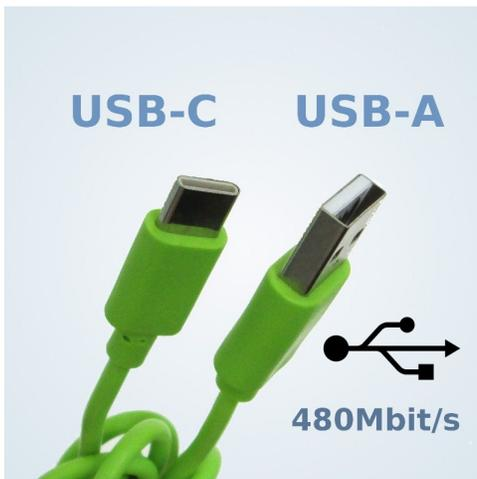
There are two varieties of USB-A to USB-C cables that allow you to plug your USB-C phone into a computer with USB-A ports. If you look closely at the “A” connector you can tell the difference. If it’s blue and/or has the 5 extra contacts, it’s capable of USB 3 speeds of 5 or 10Gbit/s; otherwise it will limit you to the USB 2 speed of 480Mbit/s. The SuperSpeed cables might have the SS trident or SS 10 trident logo on them like the amazon cable on the bottom left.
