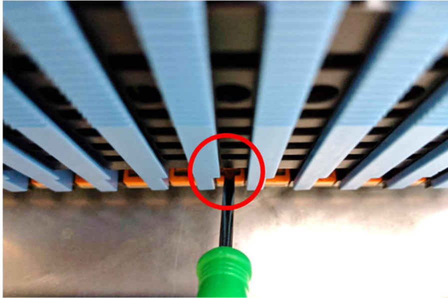
Figure 2.2 Release the latch to remove the module
